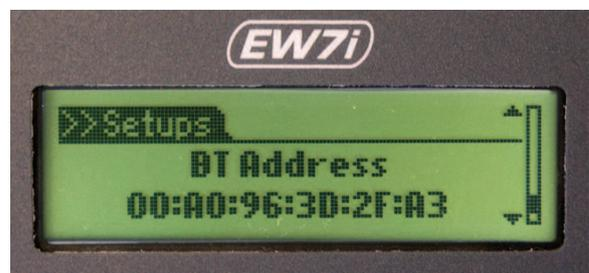
4. Push **Enter**. Use the bottom arrow to scroll down through the functions to BT Address
