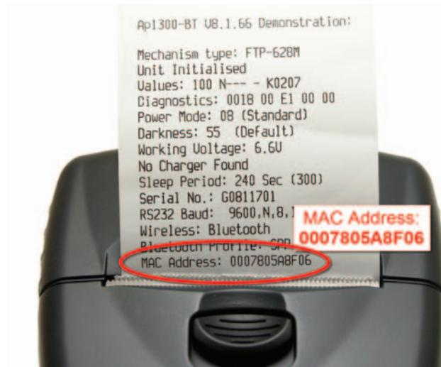
7. On the test strip, find the MAC Address. This 12 character code is the printer's Bluetooth ID.
